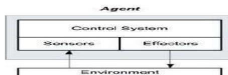
The control system provides a mapping from sensors to effectors, and provides intelligent (or rational) behavior.
